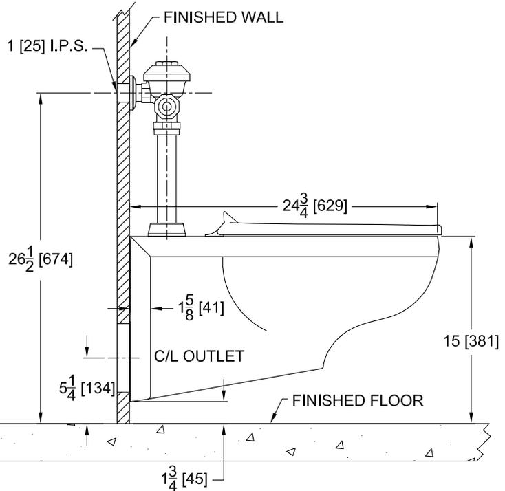
\*Note: For ADA compliance, top of seat height should be installed at 17"-19" from finished floor.
