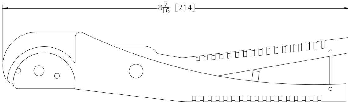
**Engineering Specification:** Zurn Tubing Cutter. Plastic bodied tubing cutter with a reversible steel blade. Cuts up to 1" ZurnPEX® tubing.
