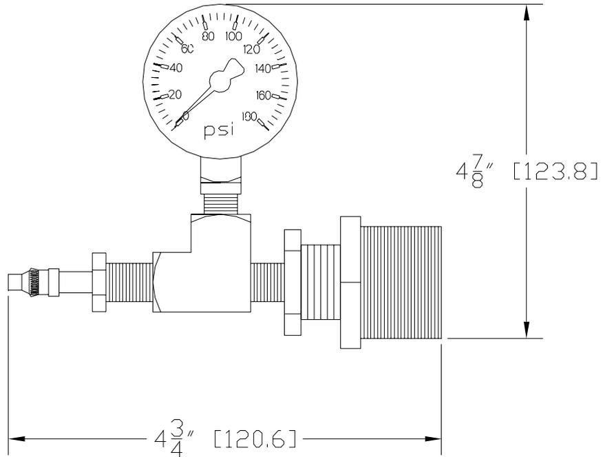
**Engineering Specification:** Zurn® air pressure test kit. Brass fittings with test gauge and schrader valve. Complete with 1" or 1-1/4" MNPT brass adapter to adapt to Zurn Radiant heating manifolds. Pressure rating up to 180 PSI.
