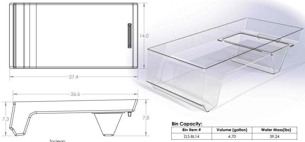
Toclean: Safe for 3 compartment sink Melting point at 410°F
