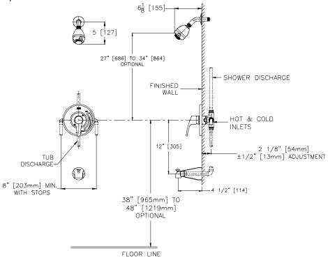
Note: All dimensions are for reference only. Do not use for pre-plumbing. Parts shown as hidden lines are supplied by others.
