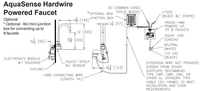
NOTE: MUST USE EITHER ZURN P6000-HW6 HARDWIRE POWER CONVERTER OR ZURN P6000-ACA PLUG-IN POWER CONVERTER TO ENSURE PROPER OPERATION. USING A POWER CONVERTER OTHER THAN ZURN MAY RESULT IN OPERATION MALFUNCTION OR UNIT FAILURE.
