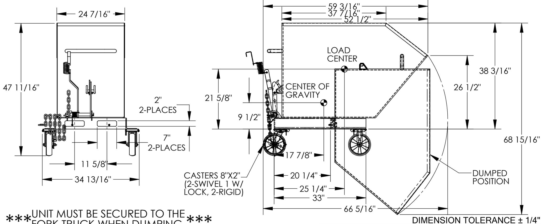
\*\*\* UNIT MUST BE SECURED TO THE FORK TRUCK WHEN DUMPING \*\*\*
