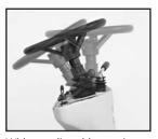
With an adjustable steering column, and heel and toe pedals for directional control, the rider sweeper provides ergonomic and safe operation.
