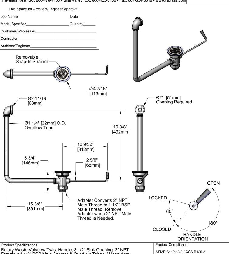
Female x 1 1/2" BSP Male Adapter & Overflow Tube w/ Head Asm.
