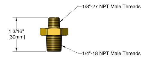
Drawn Checked **Product Specifications: KJG** Reducing Hex Nipple, 1/4"-18 NPT x 1/8"-27 NPT DMH Scale: (Unplated Brass) 1:1
