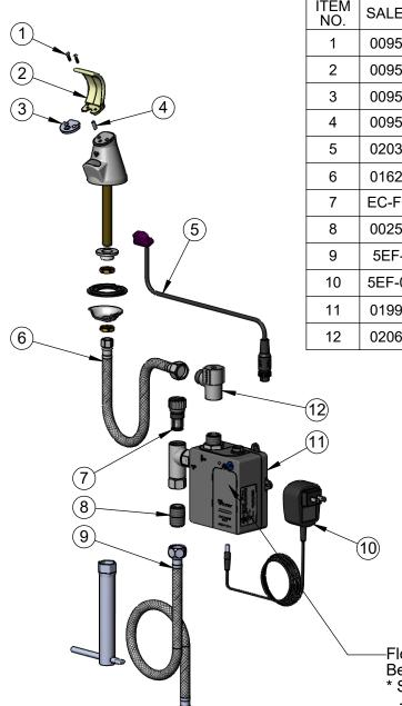
**ITEM** SALES NO. **DESCRIPTION** 009598-45 Mouth Guard Screw (2) 009595-45 Rubber Mouth Guard 009596-40 Mouth Guard Holder 009594-45 Flow Straightener Sensor Cable Assembly - Curved Lens 020315-45 Inlet Hose, Faucet, 1/2" NPSM-F x 1/4" NPSM-F 016297-45 **EC-FILTER** Replacement Filter Close Nipple, 1/2" NPT 002534-25 Supply Hose, 9/16-24 Female x 1/2" NPSM 5EF-0005 5EF-0002C AC Adapter - US Plug 019944-45 ChekPoint Control Module w/ Filter Tee 020672-40 Flow Control Valve
