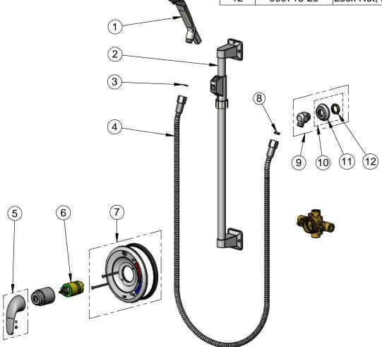
Product Specifications: Pressure Balance Shower Valve (ASSE 1016), Shower Queen Handheld Spray Assembly and Vertical Assist Bar
