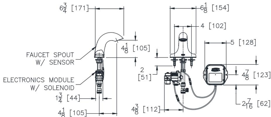
*Note: Endpoint must be installed within a 2' [610] radius of faucet.*
