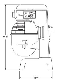
**MACHINE ELECTRICAL SPECS:** 120/60/1 - ETL Listed
