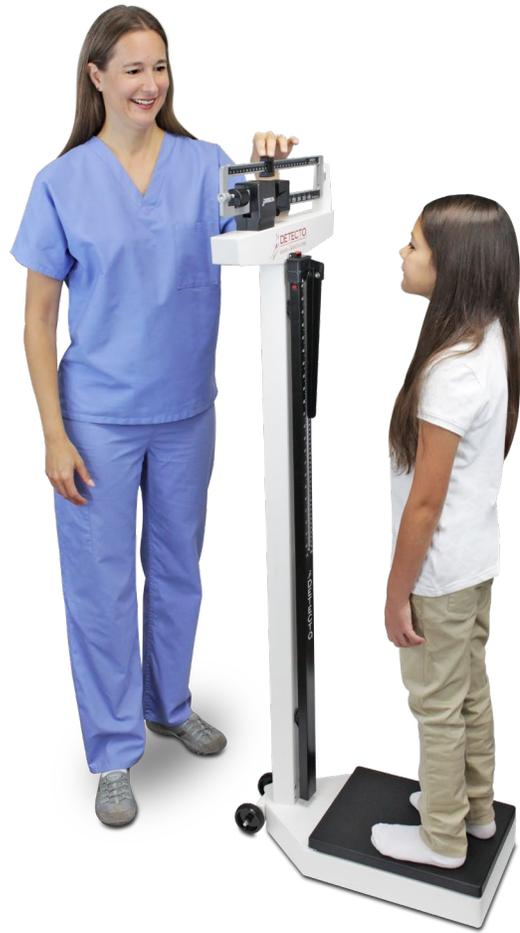
When the patient steps on the scale, simply move the large poise and then the small poise until the weighbeam balances. It's that simple!
