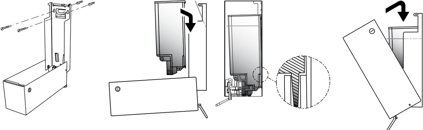
1. Mount dispenser to wall using enclosed screws and wall plugs.
