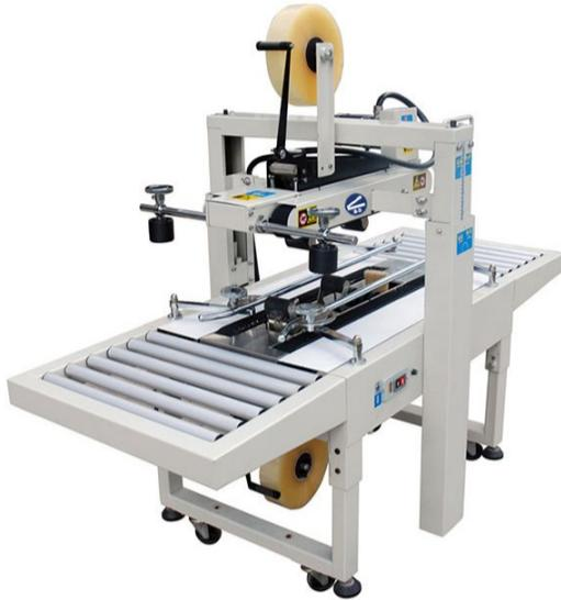
The **CS-6050 Semi-Automatic Uniform Carton Sealer with Easy Manual Carton Size Adjustment** has a 4-belt design (2 top and 2 bottom). The machine comes complete with infeed / exit conveyors, casters, power cord and plug.
