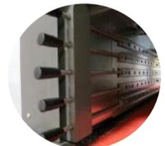
Adjustable Air Flow Dampeners to Concentrate Air Flow to Specific Locations on Package
