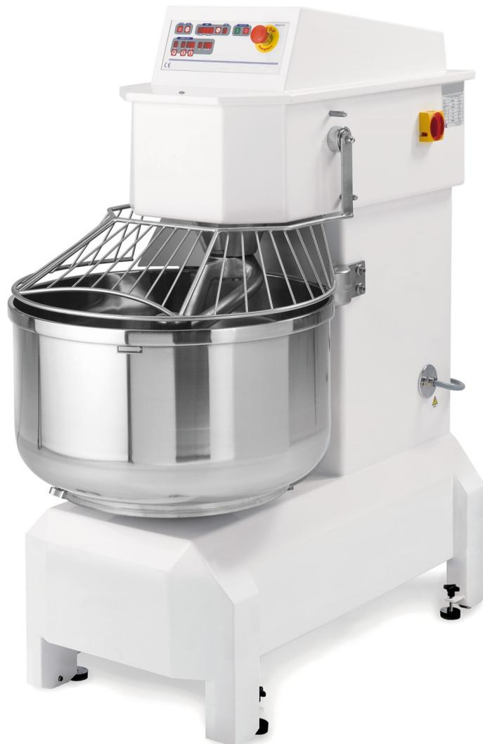
**Spiral Mixer, 175 Lb. Dough Capacity, 2 Speeds, Programmable Digital Control, Stationary Stainless Steel Bowl, Safety Guard & Dough Hook, Cast Iron Frame with Enamel Coated Steel Finish, 7 HP, 208-240/60/3P/20A, NEMA 15-30P**
