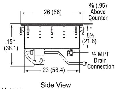
\*Manifold drain adds 6 1/2 (16.5) to overall height
