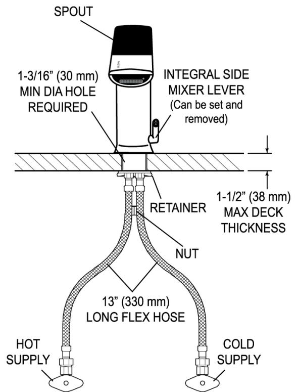
Solenoid carrier includes strainer for easy above deck service. Thermostatic mixer ordered separately to comply with ASSE 1070 requirements. The product shall be tested and certified to industry standards: ASME A112.18.1M, CSA B125.1, California Health and Safety Code 116875
