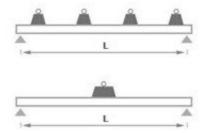
The maximum weight load is based on an evenly distributed weight load between 2 points
