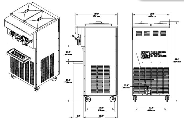
Minimum Wall Clearance Both Sides and Back -6 inches (152 mm)
