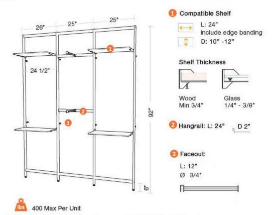
The max weight load is based on an evenly distributed weight load.
