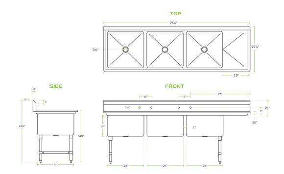
NSF Listed 16 Gauge Galvanized Steel Stainless Steel 3 Compartments 1 Drainboard Type 304 1 Drainboard Straight / Line Sinks
