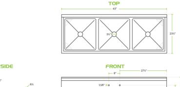
NSF Listed 16 Gauge Galvanized Steel Stainless Steel 3 Compartments None Type 304 0 Drainboards Straight / Line Sinks
