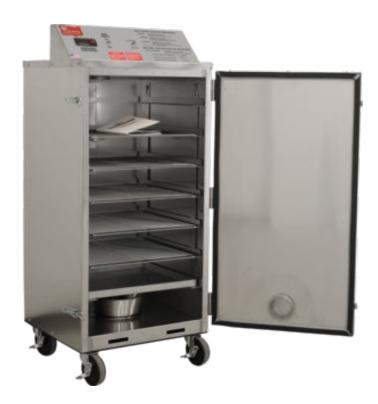
Constructed with 304 grade stainless steel, double walled with 18ga interior thickness with 850 degree high temperature spin glass insulation for maximum heat retention.
