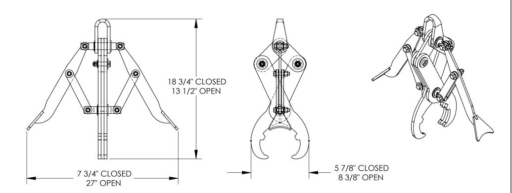
NOTE: OVERALL DIMENSIONS GIVEN IS THE MAX/MIN FOR EACH VALUE
