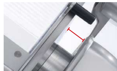
Increased gap between blade and machine body
