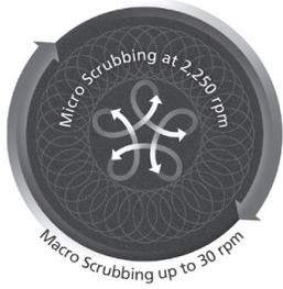
Patented REV™ random orbital scrubbing technology with high speed ¼ inch micro scrubbing and 14 inch rotational macro scrubbing attacks dirt from multiple directions for superior cleaning effectiveness.
