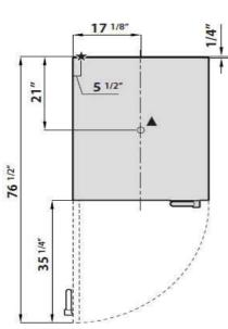
★ Main power cable▲ Drain pipe ø 31
