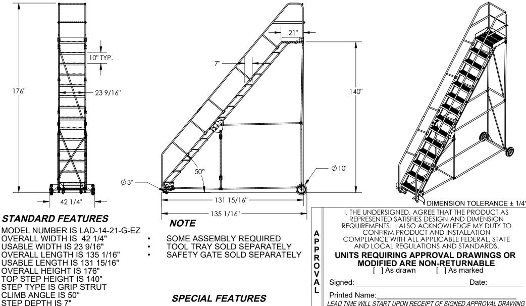
TOP STEP DEPTH IS 21" NONE MAX CAPACITY IS 350 LBS WHEEL SIZE IS Ø10" FRONT WHEEL SIZE IS Ø 3" TOUGH BAKED IN POWDER COATED BLUE FINISH
