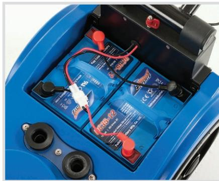
Maintenance-free AGM batteries and onboard charger.
