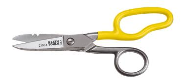
These Scissors are free-fall snips that feature stainless steel blades for blade sharpness and durability. They cut 19 AWG and 23 AWG electrical communication wire, cable and cordage. The extended handle allows for more comfortable cutting and provides leverage during wire cutting. The free-fall design makes this snip easier to use.
