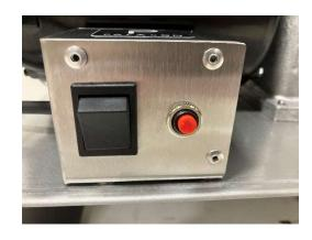
Easy to use controls include an on/off rocker switch and push button reset button
