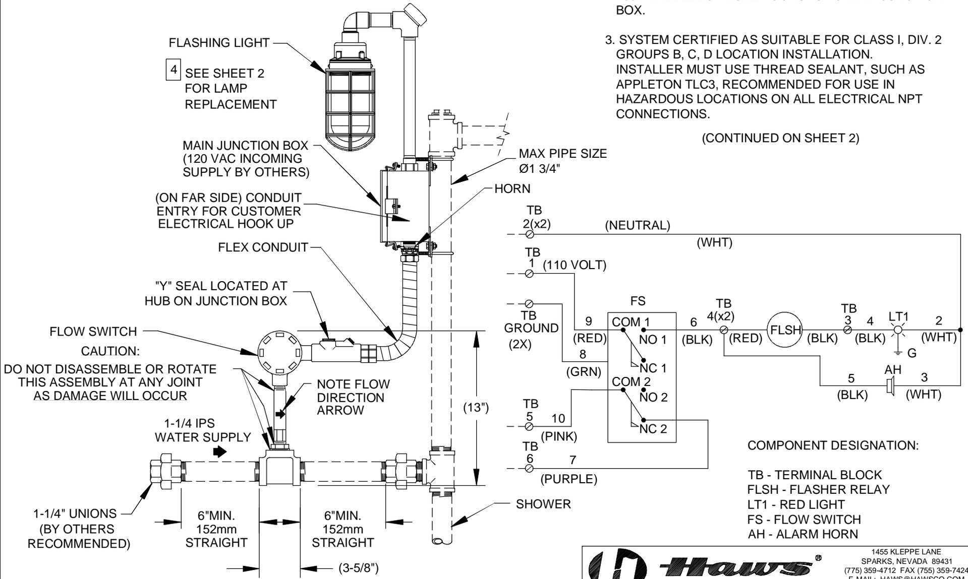
**SWITCH MUST BE MOUNTED IN HORIZONTAL POSITION**
