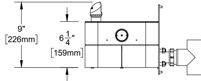
NOTE: STANDARD CONFIGURATION FOR MODEL 3670 ON A PEDESTAL IS SHOWN. IT IS RECOMMENDED THAT THE ASSEMBLY IS PLACED AT THE LOWEST OPENING ON THE PEDESTAL. THE MOUNTING PLATE CAN BE ROTATED SO THE DOG BOWL CAN BE IN A "HIGH" OR "LOW" POSITION. IT IS RECOMMENDED TO USE THE "LOW" POSITION AS SHOWN.
