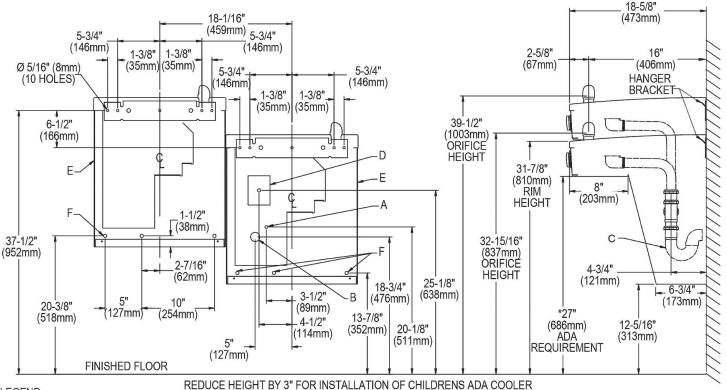
A = Recommended water supply location. Shut off valve (not furnished) to accept 3/8" O.D. unplated copper tube. 3" (76mm) maximum out from wall.
