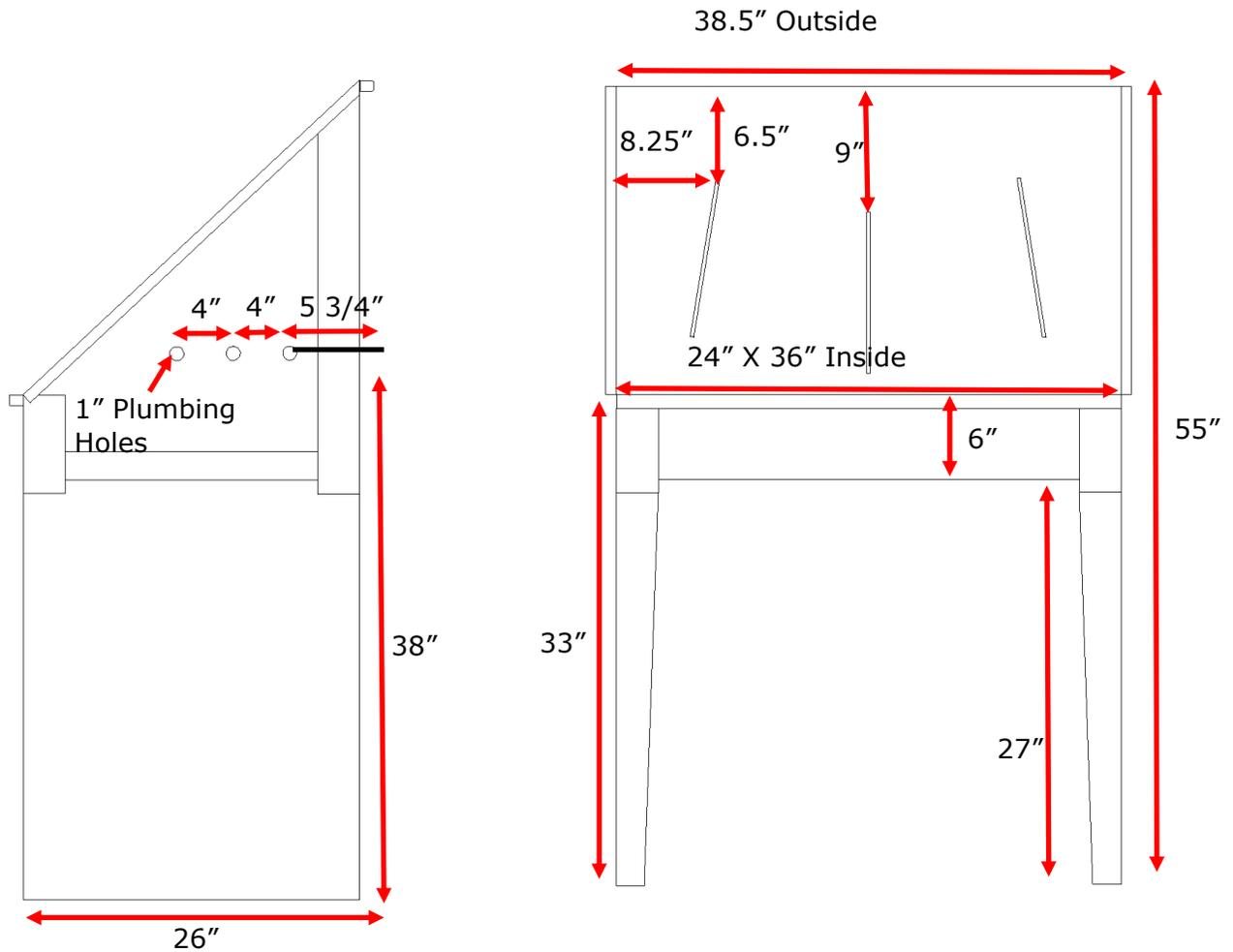
Available as Left, Right or center drain. 3.5" drain hole, located 7" on center from the left or right.
