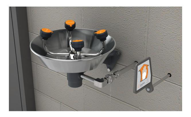
**Application:** Freeze-resistant WideArea<sup>™</sup> eye/face wash for wall mounting. Valve and supply line are located behind wall in heated area to prevent freezing. Self-draining valve permits water to drain completely from unit after use. Since unit is intended for use in cold weather conditions, consideration should be given to supplying unit with tempered water in accordance with ANSI Z358.1-2014. See "Tempering Valves" section for more information.
