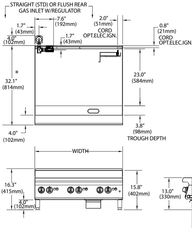
For use with Natural or Propane gas only. Gas input ratings shown for installations up to 2000 ft., (610m), above sea level. Please specify altitudes over 2000 ft. and gas type required when ordering.
