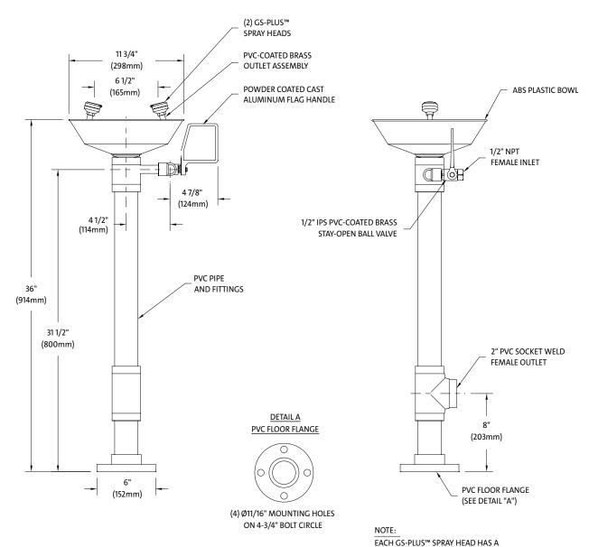
"FLIP-TOP" DUST COVER, INTERNAL FLOW CONTROL AND FILTER TO REMOVE IMPURITIES FROM THE WATER FLOW.
