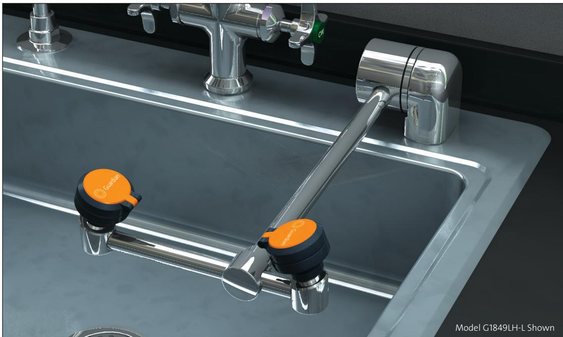
**Application:** AutoFlow™ eyewash for mounting on counter. Spray heads swing down from storage to operational position, activating water flow. Available in a variety of spray head configurations to minimize obstructions at a sink. *Note: If unit is not installed at a sink, floor drain should be provided underneath unit to prevent accumulation of water on floor.*
