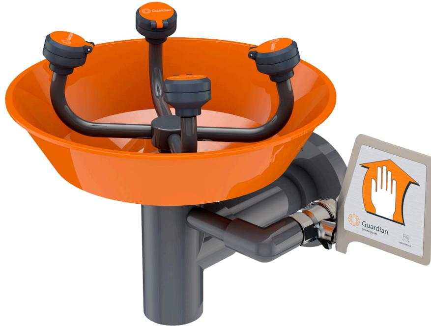
**Application:** WideArea™ eye/face wash for wall mounting. Unit is constructed of PVC, PVC-coated components and a stainless steel valve for superior corrosion resistance. Ideal for use in industrial environments where harsh acids or caustics are present. Four GS-Plus™ spray-type outlet heads deliver a flood of water over a wide area of coverage for complete rinsing of eyes and face.
