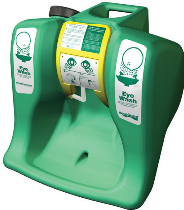
**Application:** Self-contained 16 gallon gravity-flow eyewash unit is ideal for use in low traffic areas, and where a continuous supply of potable water is unavailable for plumbed units. Rugged plastic tank is wall mountable near any hazard. Unit uses gravity to deliver approximately eight gallons (30 liters) of water for 15 minutes through dual spray heads, thus complying with the provisions of ANSI Z358.1-2014 for eyewashes.
