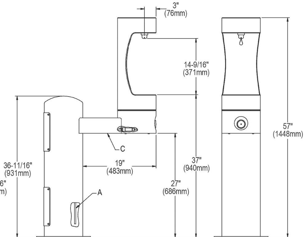
A = 3/8" O.D. Unplated copper tube connect. Shut off valve by others.
