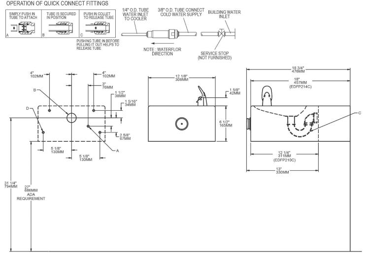
A = Recommended water supply location 3/8" (10mm) O.D. unplated copper tube connect stub 1-1/2" (38mm) out from wall - shut off valve by others. B = Recommended location for waste outlet 1-1/4" (32mm) O.D. drain stubbed 6-5/8" (168mm) from the wall. C = 1-1/4" (32mm) trap not furnished.
