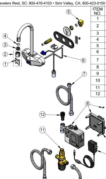
DESCRIPTION SALES NO. 015425-45 Vandal Resistant Key 0.5 GPM VR Non-Aerated Spray B-0199-06-N05 Device, 55/64-27 Female 044A 3/8" to Aerator Adapter 006575-45 O-Ring 015345-20 Low Profile Elbow, 3/8 NPSM 017195-45 Angled Sensor with Cable Flexible Connector Hose, 3/8" NPSM x 016325-45 1/2" NPSM 016647-45 ChekPoint Control Module (Grey) 5EF-0002 A/C Transformer Supply Hose, 9/16-24 Female x 1/2" 5EF-0005 NPSM EC-TMV ASSE 1070 Thermostatic Mixing Valve **EC-FILTER** Replacement Filter
