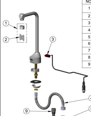
ITEM DESCRIPTION SALES NO. NO. VR 1.5 GPM Laminar Flow Device (Anti-Microbial) B-0199-06-LF15A w/ VR Key 015425-45 Vandal Resistant Key 019174-45 Sensor Cable Assembly 016297-45 Inlet Hose, Faucet, 1/2" NPSM-F x 1/4" NPSM-F ChekPoint Control Module w/ Filter Tee 019944-45 5EF-0002C AC Adapter - US Plug 5EF-0005 Supply Hose, 9/16-24 Female x 1/2" NPSM 002534-25 Close Nipple, 1/2" NPT **EC-FILTER** Replacement Filter
