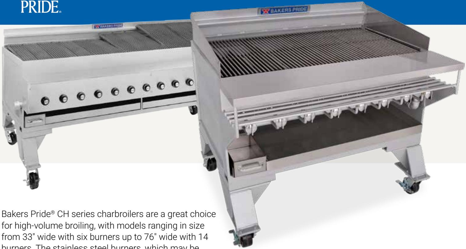
Bakers Pride® CH series charbroilers are a great choice for high-volume broiling, with models ranging in size from 33" wide with six burners up to 76" wide with 14 burners. The stainless steel burners, which may be substituted for cast iron, each have an output of 18,000 BTUH for energy efficiency yet high production
